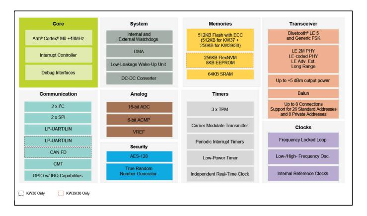
View additional information for KW39/38/37: 32-Bit Bluetooth 5.0 Long-Range MCUs with CAN FD and LIN Bus Options, Arm® Cortex®-M0+ Core.
