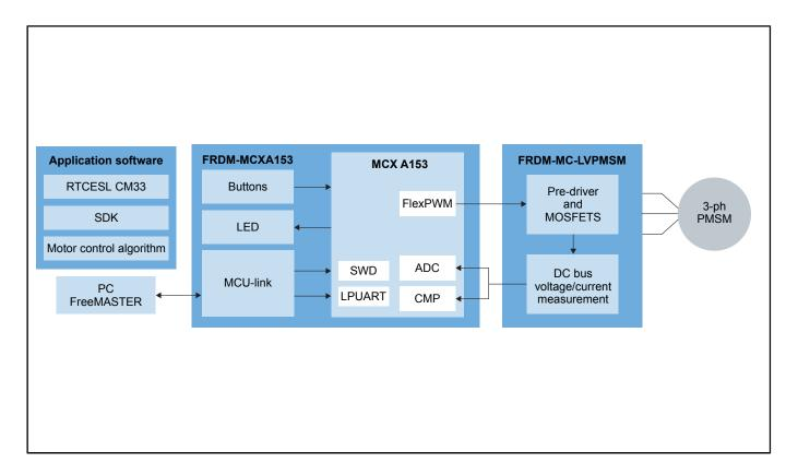
View additional information for PMSM Sensorless FOC Using MCX A153.
