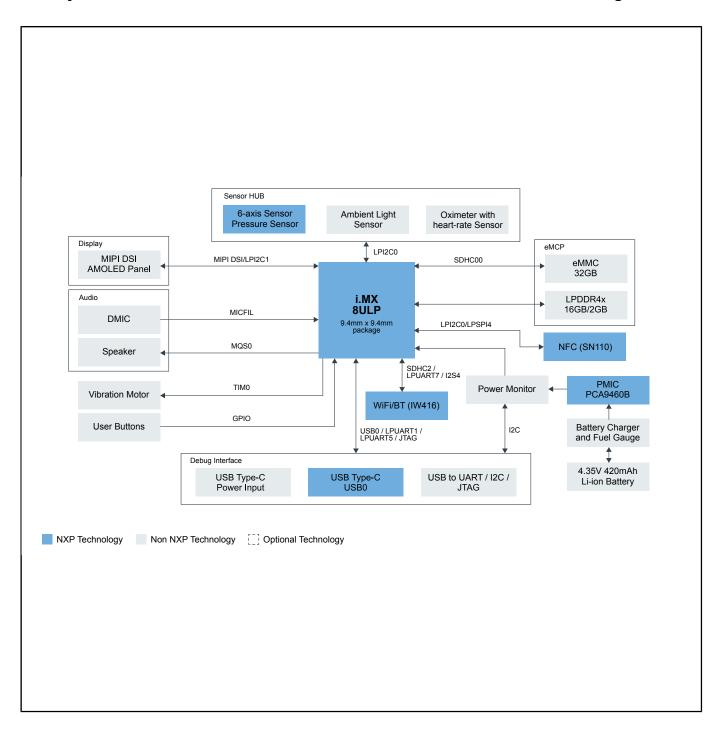
View additional information for Battery Powered Portable Device Design Based on i.MX 8ULP.
