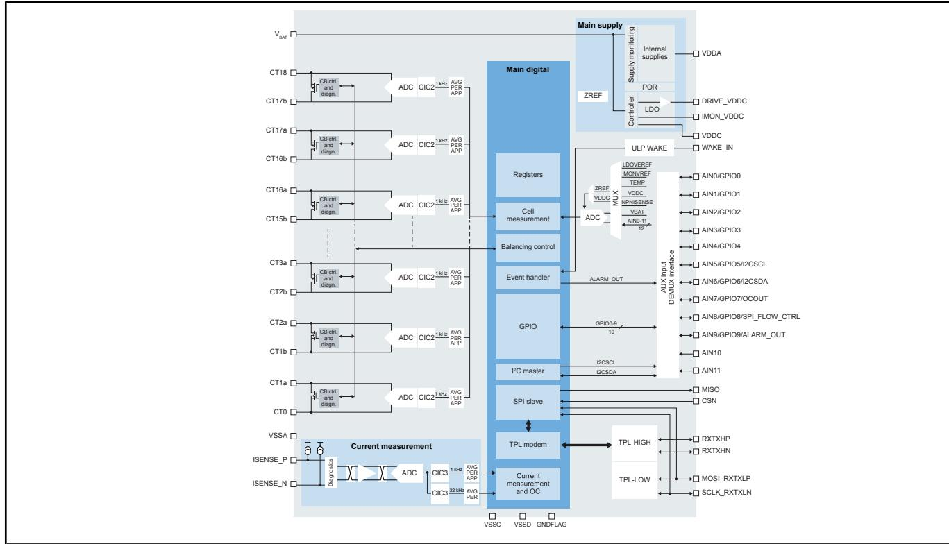
[View additional information for 18-Channel Li-Ion Battery Cell Controller IC.](#)
