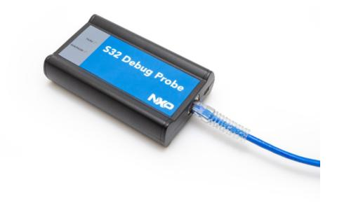
**Note:** When you configure the debugger for the hardware connection, you will need to specify the S32 Debug Probe IP address or hostname. The CCS findcc utility is used to search any probe on the local subnet. For more information, see Using CCS to search for S32 Debug Probes on page 27 topic.
