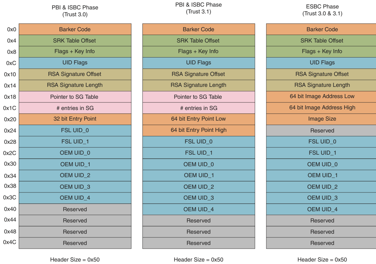
Figure 35. CSF header structure
