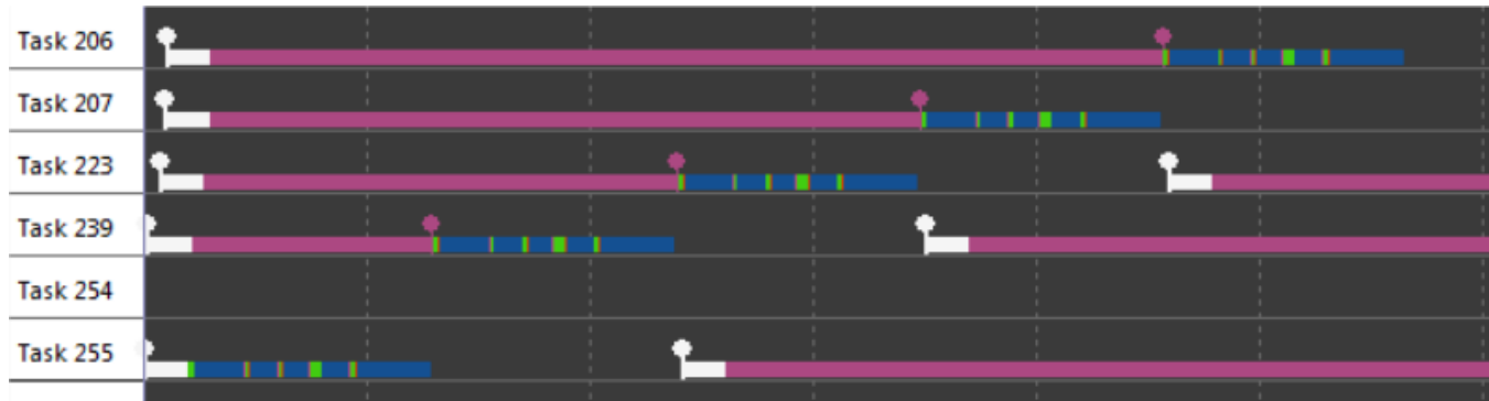
Figure 186. Tasks Executing Sequentially
