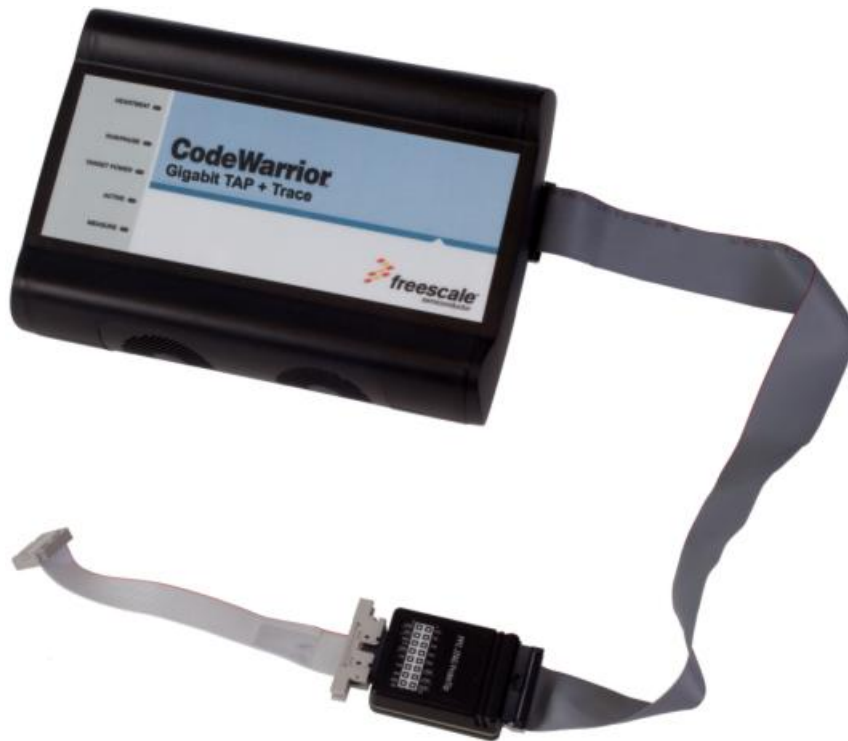
Figure 3-3. Flexible probe tip extension cable attached to JTAG/COP header
