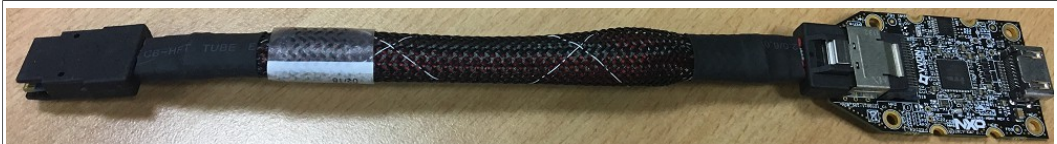
Figure 3. i.MX mini SAS cable with LVDS-to-HDMI adapter
