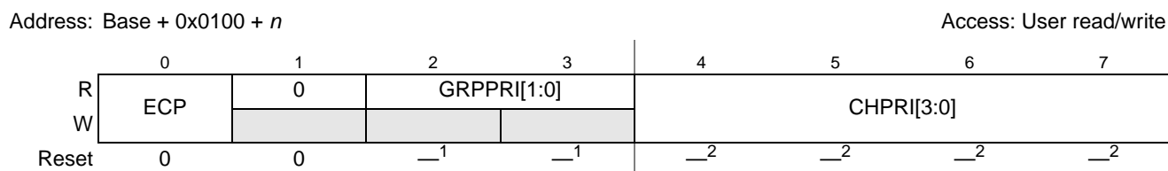
Figure 9-21. DMA Channel n Priority Register (DCHPRI n )
