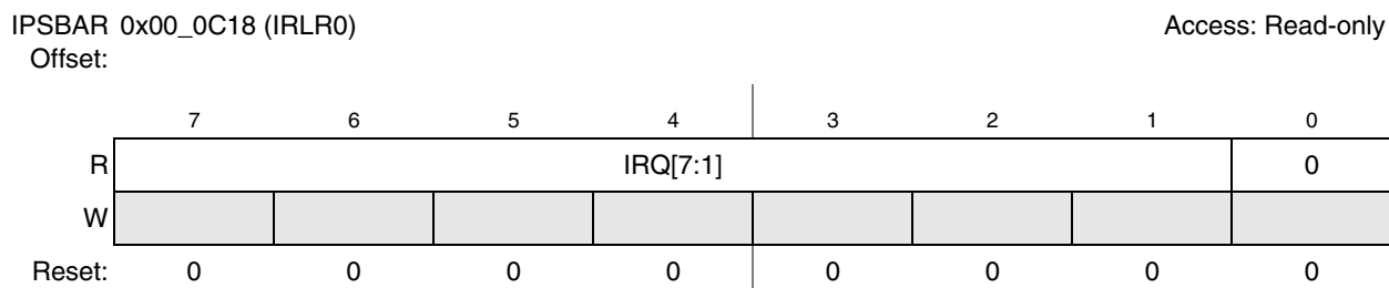
Figure 15-7. Interrupt Request Level Register (IRLR n )
