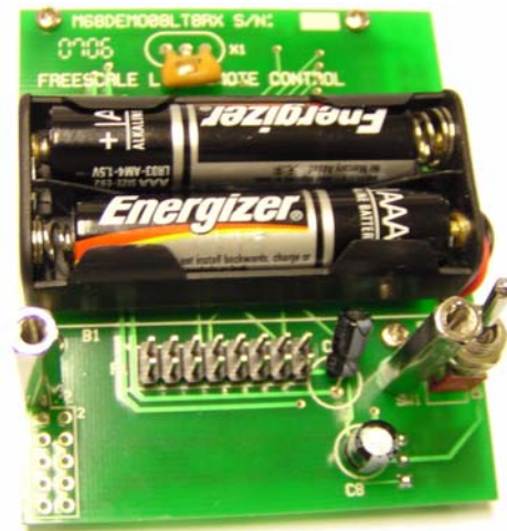
(b) Back of IR RC Receiver
