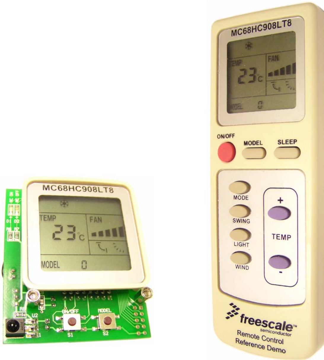
(a) MC68HC908LT8 IR RC Receiver
