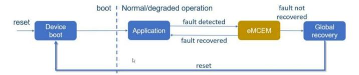
Figure 5. eMCEM (Extended Microcontroller Error Manager)
