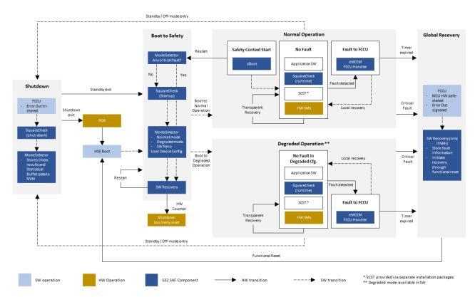
Figure 3. S32 Safety Software Framework operation diagram
