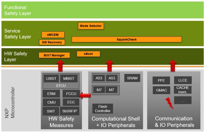
Figure 2. NXP's Safety Software Framework content
