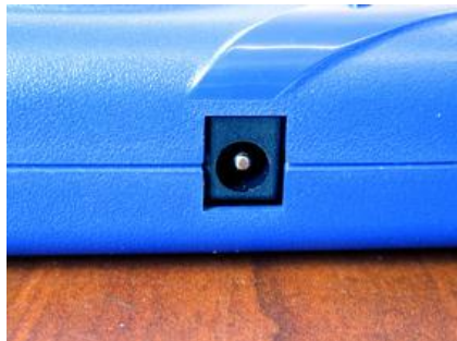
Figure 16. Power Jack for Connecting 6V DC Supply – Cyclone Pro
