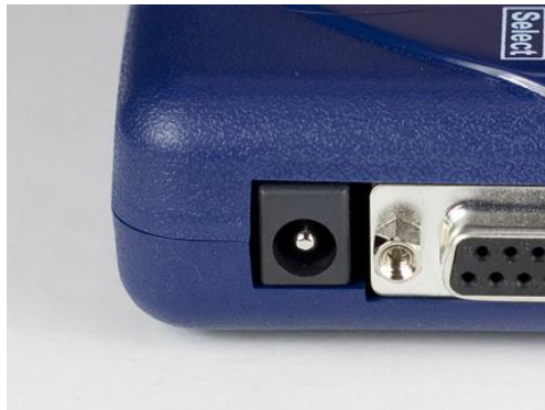
Figure 20. Power Jack for Connecting 6V DC Supply – Cyclone for ARM® Devices
