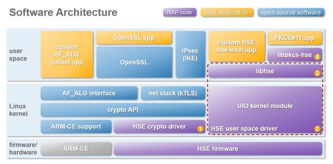
Figure 1. Linux crypto architecture
