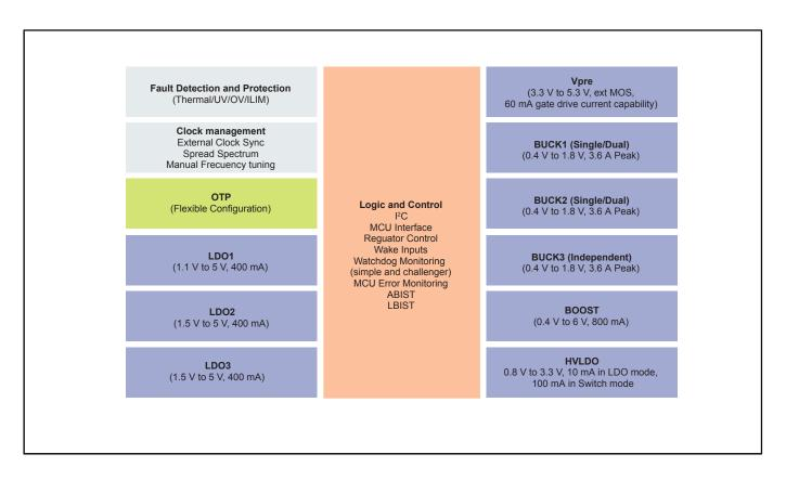
View additional information for Multi-Channel (9) PMIC for S32G Processor – 8 High Power, 1 Low Power, Fit for ASIL D Safety Level.
