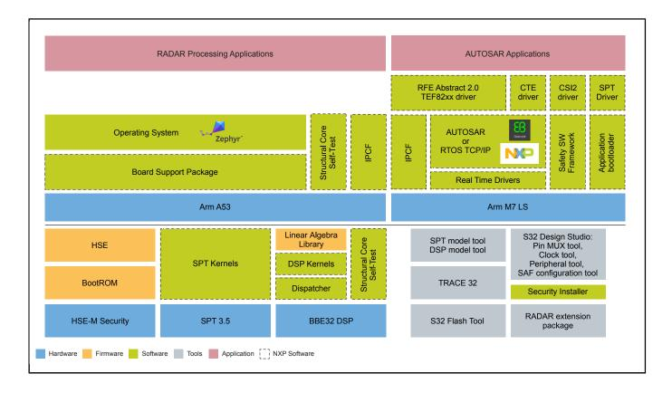
View additional information for S32R41 High-Performance Processor for High-Resolution Radar.
