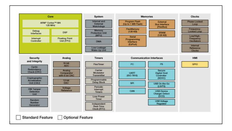
View additional information for Kinetis K21-120 MHZ, Full-Speed USB, Anti-Tamper Microcontrollers based on Arm® Cortex®-M4.
