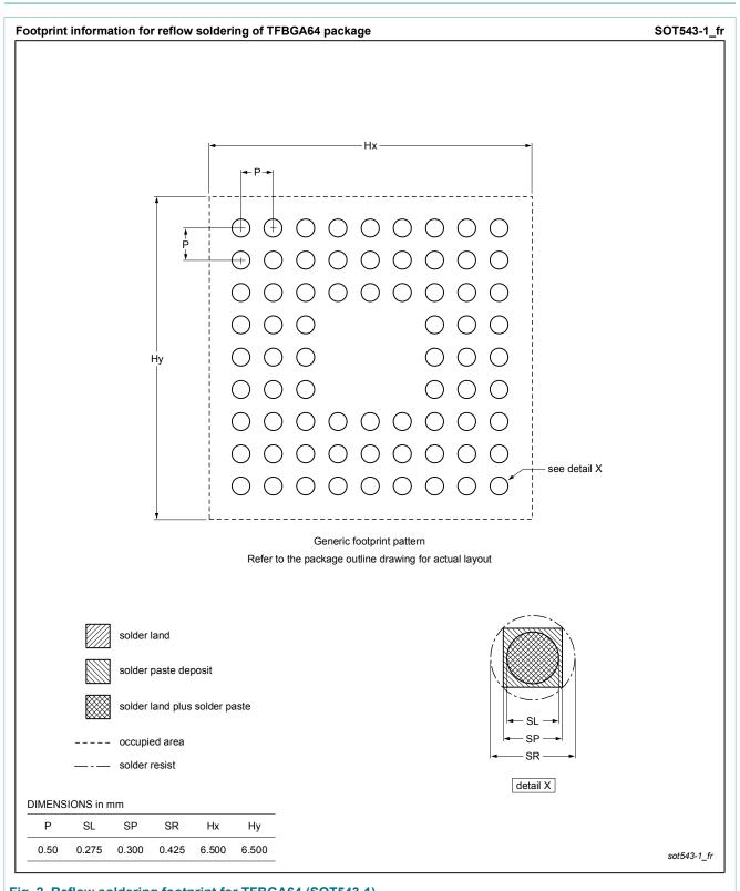
Fig. 2. Reflow soldering footprint for TFBGA64 (SOT543-1)
