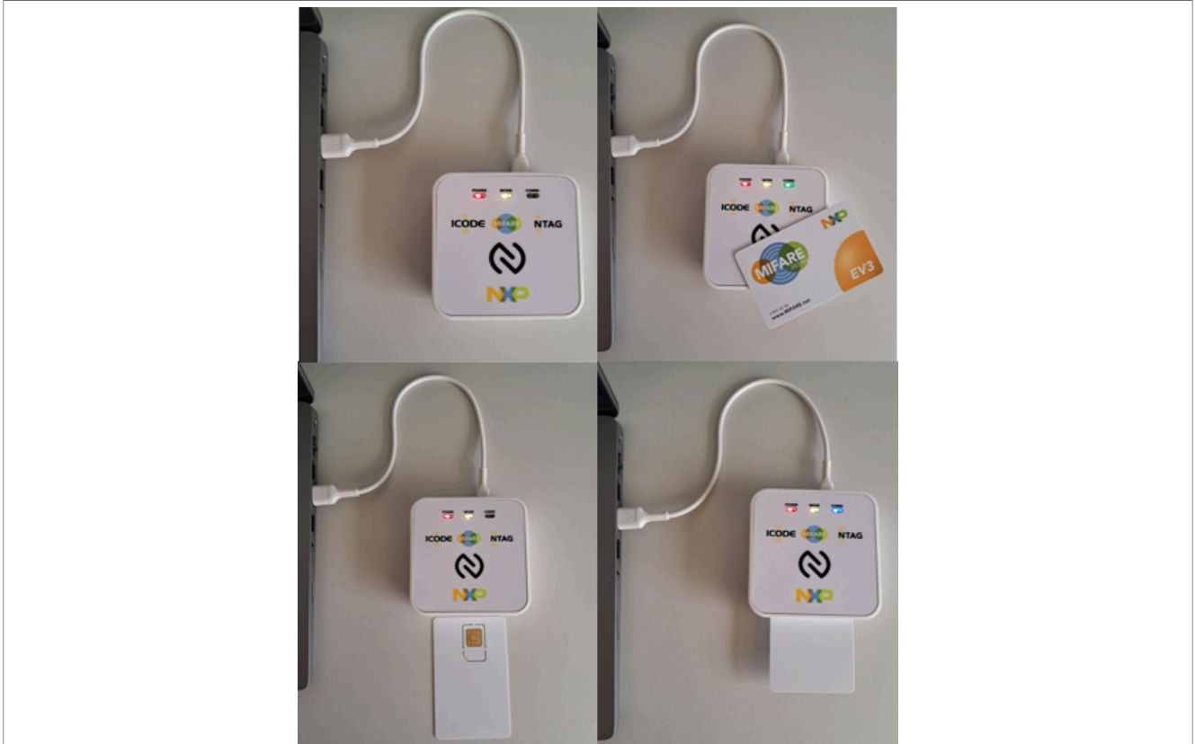
Figure 9. Aspect of Pegoda leds when in default (PS/SC) mode. Presence of card both in contactless interface as well as in contact interface turns COMM LED from off to colored green
