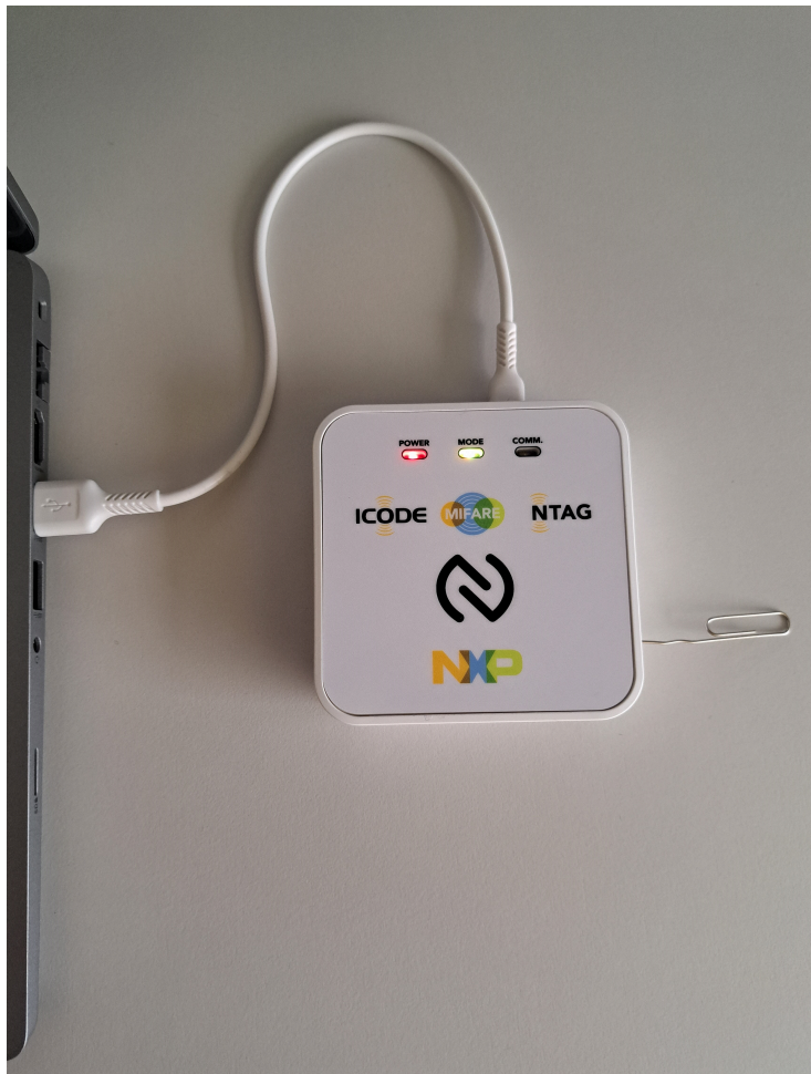
Figure 15. Pegoda has a lateral access to an internal PCB pushbutton: while in PS/SC, pressing this button toggles VCOM mode with PC/SC mode.
