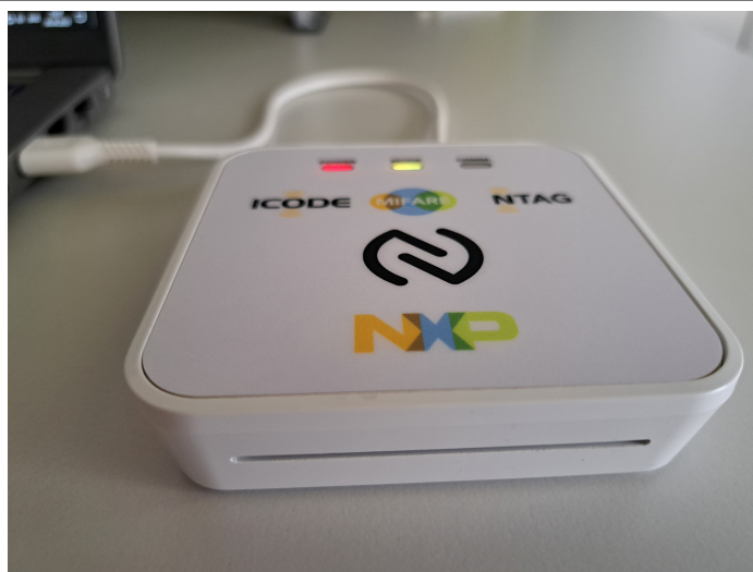
Figure 5. Frontal aspect of Pegoda CLRD730, showing ISO/IEC7816 slot and contactless antenna near NXP logo
