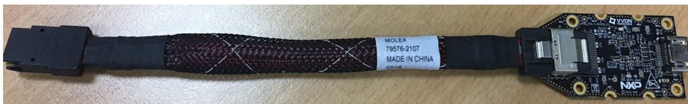
Figure 14. i.MX mini SAS cable with DSI-to-HDMI adapter
