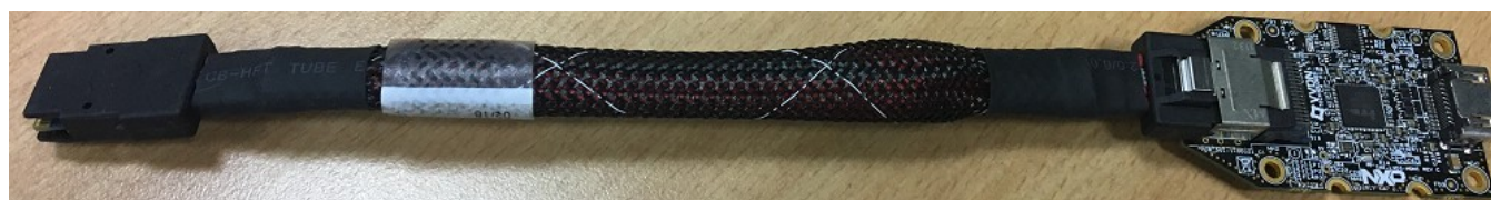
Figure 20. i.MX mini SAS cable with LVDS-to-HDMI adapter
