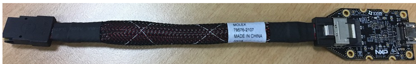
Figure 19. i.MX mini SAS cable with DSI-to-HDMI adapter
