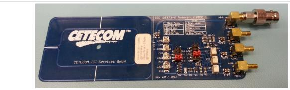
1. The jumper settings allow the use of different pre-calibration settings.
