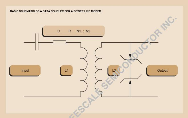
In the above figure, values of R, C and the ratio of the transformer depend on the actual data rate and power and frequency of the signal. For use in frequencies ranging from 95 kHz to 148.5 kHz, the coupled signal of age can reach up to 116 dBµ\( \) aling 631 mV.
