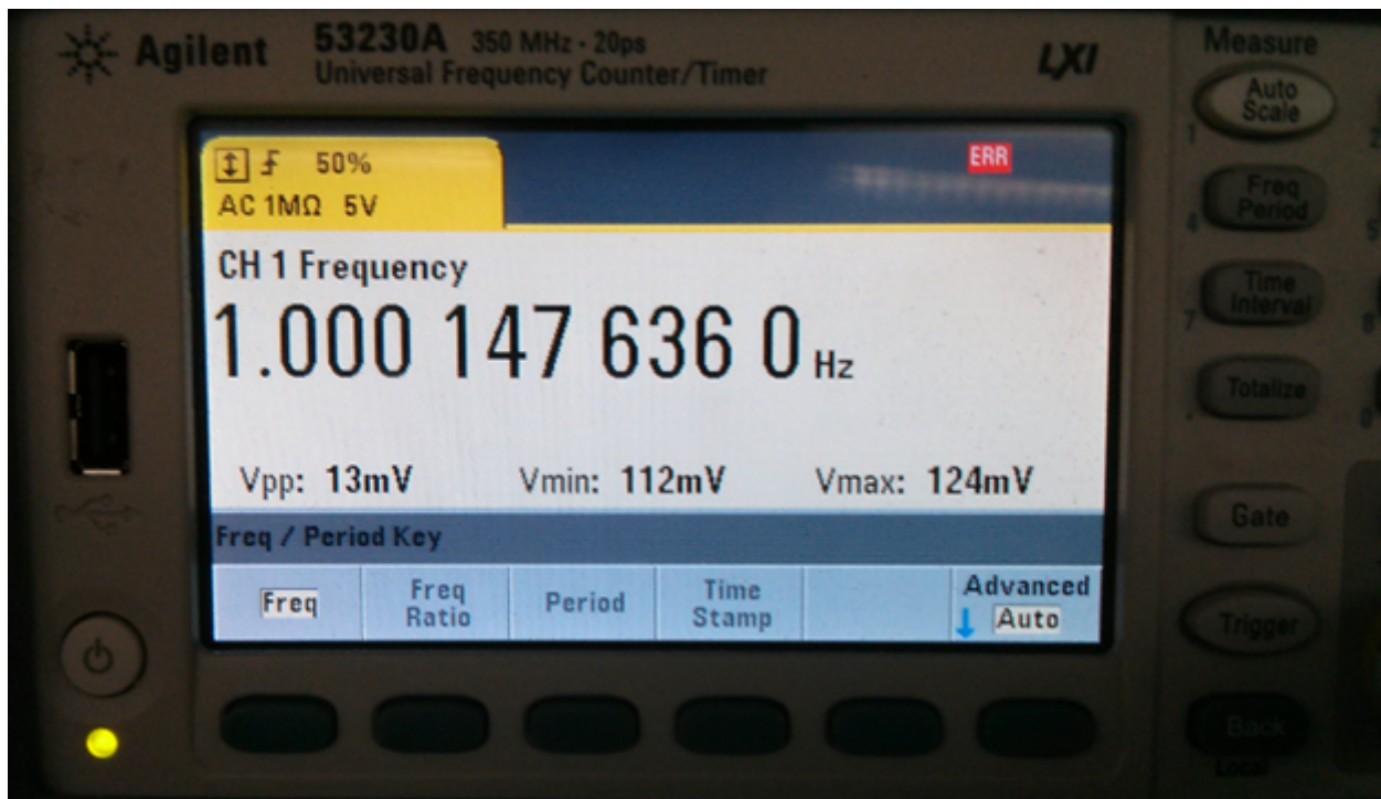
Figure 2. Output with uncorrected crystal error
