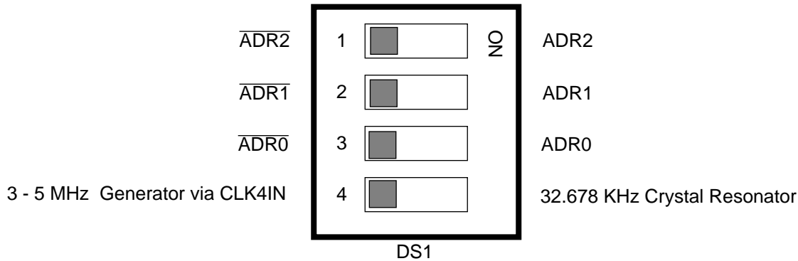
FIGURE 2-2 Configuration Dip-Switch - DS1
