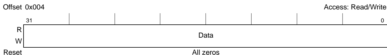
Figure 17-13. PCI Express Configuration Data Register (PEX_CONFIG_DATA)
