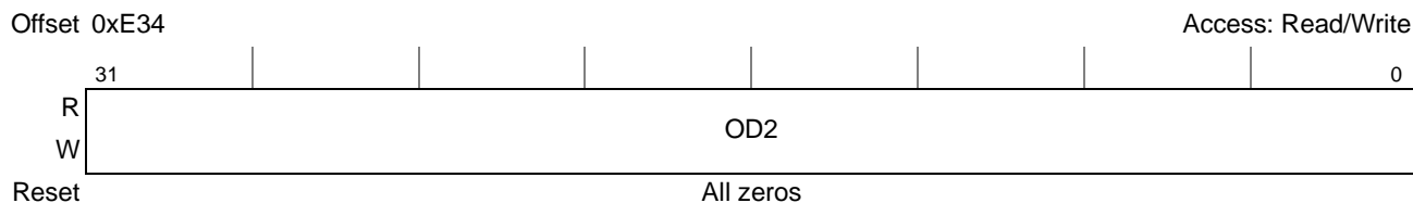
Figure 17-45. PCI Express Error Capture Register 3 (PEX_ERR_CAP_R3) Internal Source, Outbound Transaction
