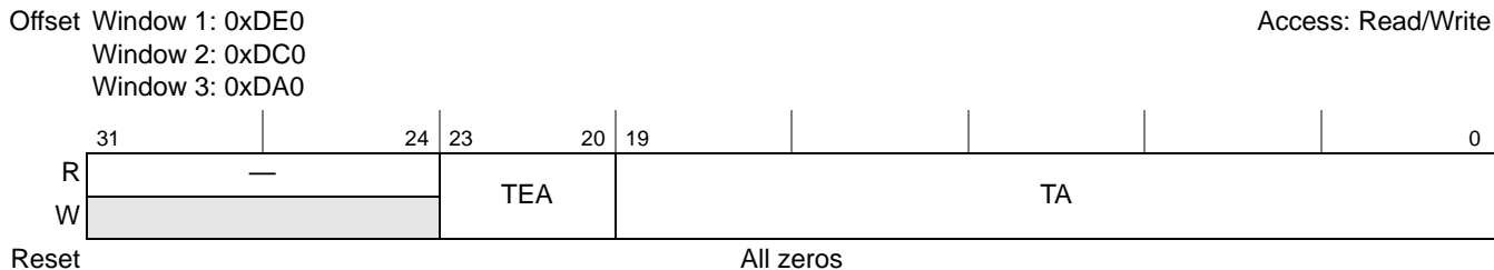
Figure 17-34. PCI Express Inbound Translation Address Registers (PEXITAR n )
