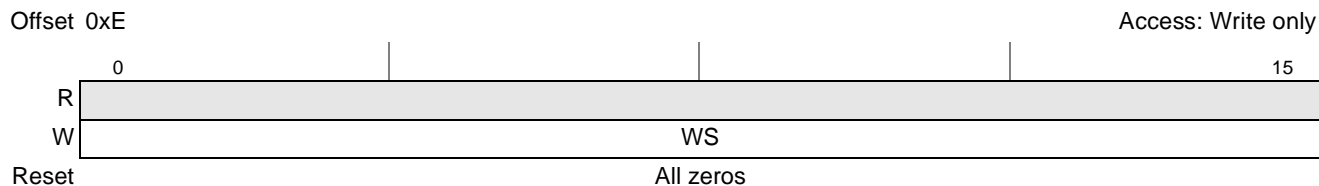
Figure 5-30. System Watchdog Service Register (SWSRR)
