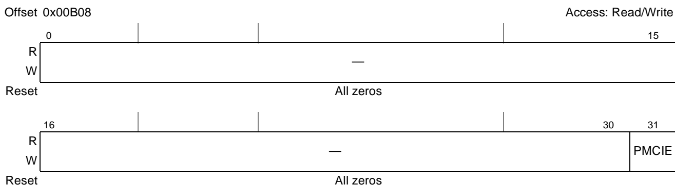
Figure 5-62. Power Management Controller Mask Register
