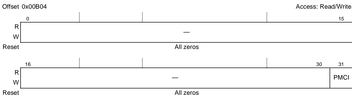
Figure 5-61. Power Management Controller Event Register
