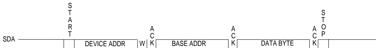
Figure 16-126. Byte Write to Device with Internal Addresses
