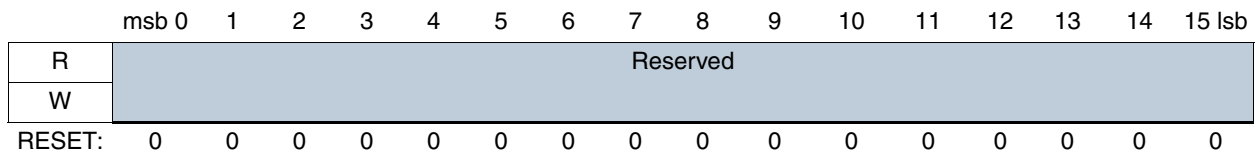
Figure 49. Codec Clock Register (MBAR + PSCx + 0x20)—CCR for Other Modes for Prior Versions of the MPC5200
