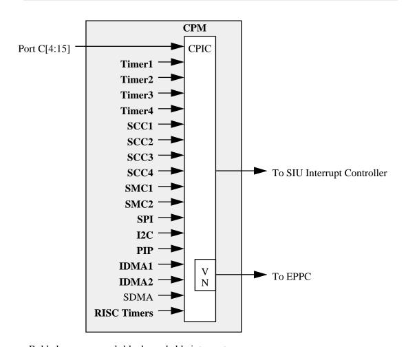
Bolded names are sub-block maskable interrupt sources.
