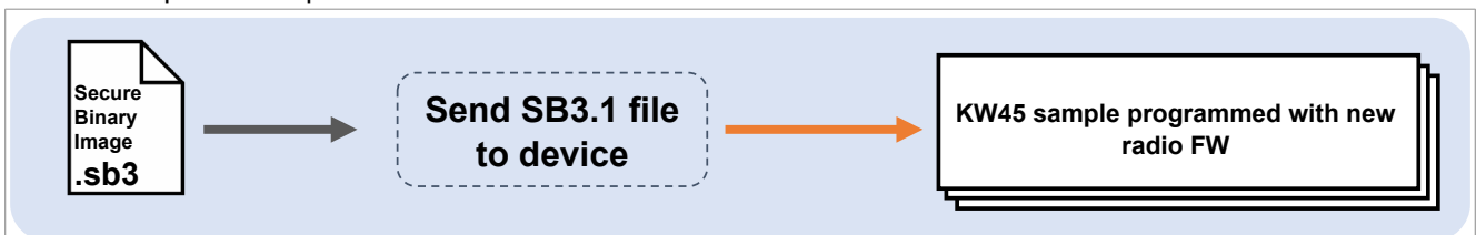
Figure 14. In this step, the generated *.sb3 file is programmed in KW45
