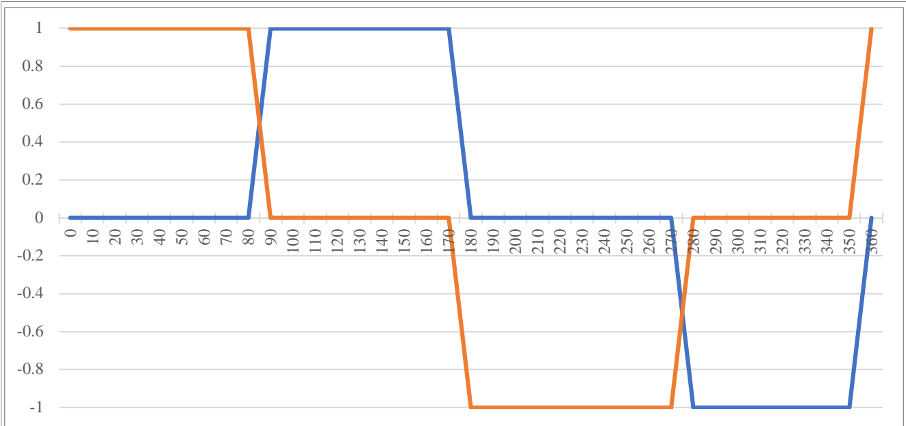
Figure 4. Single phase step control timing
