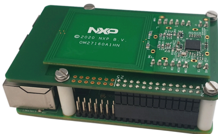
Figure 11. OM27160 Development kit + Raspberry Pi connected
