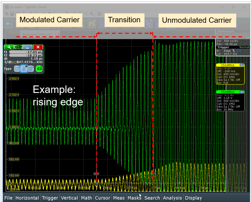
Figure 4. PN5190 TX shaping principle
