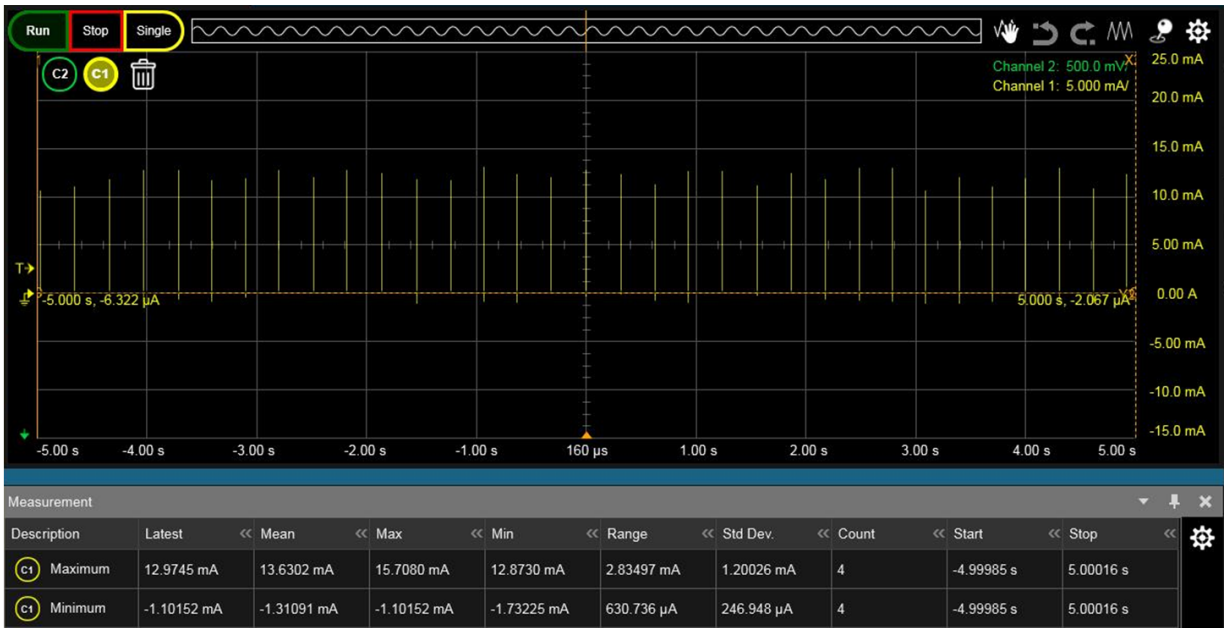
Figure 34. KW36 current consumption in low-pwoer mode 1 with a coin cell
