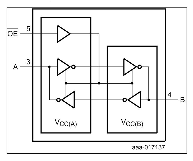
View additional information for Dual-Supply Translating Transceiver (Auto-Direction Sensing, Three-State).
