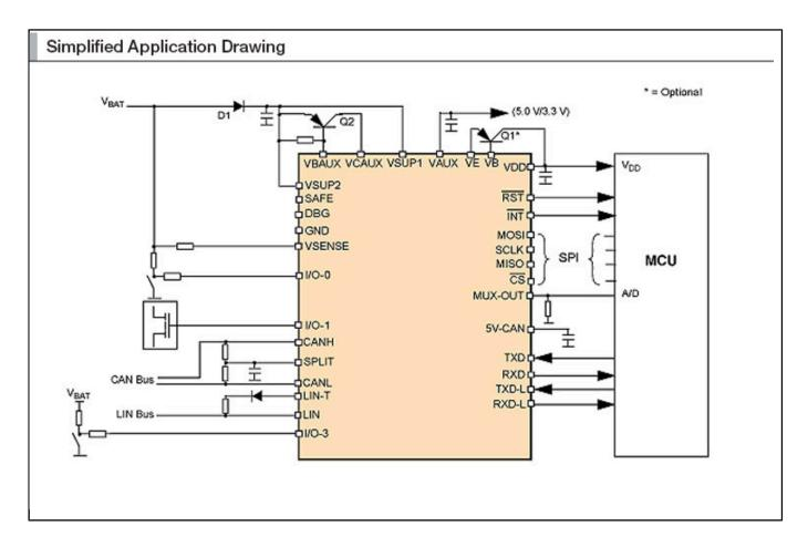
View additional information for System Basis Chip with CAN High-Speed and LIN Interface.
